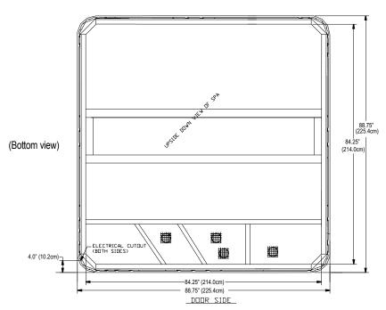
**NOTE:** Watkins Manufacturing Corporation recommends that the Tempo be installed on a minimum 4" thick reinforced concrete pad or structurally sound deck able to support the "dead weight" found in the spa specification chart.
