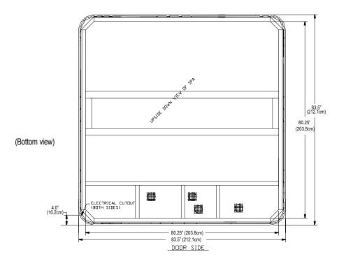
**NOTE:** Watkins Manufacturing Corporation recommends that the Relay be installed on a minimum 4" thick reinforced concrete pad or structurally sound deck able to support the "dead weight" found in the spa specification chart.
