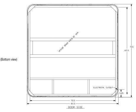
**NOTE:** Watkins Manufacturing Corporation recommends that the Trinidad be installed on a minimum 4" thick reinforced concrete pad or structurally sound deck able to support the "dead weight" found in the spa specification chart.
