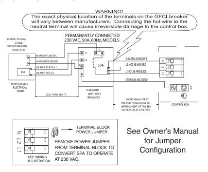
Your spa contains a control box designed to operate at 230V, 60Hz. Installation of a 50 amp. dedicated circuit is required. The control box must be hard wired directly to a subpanel protected by a Ground Fault Circuit Interrupter (GFCI). The subpanel containing GFCI breakers is included with the spa.
