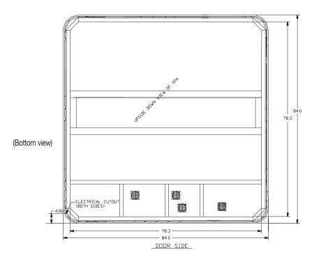
**NOTE:** Watkins Manufacturing Corporation recommends that the Mallorca be installed on a minimum 4" thick reinforced concrete pad or structurally sound deck able to support the "dead weight" found in the spa specification chart.
