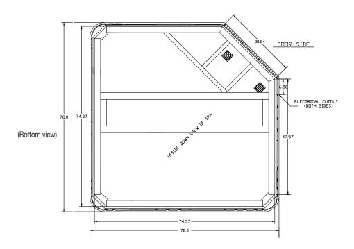
**NOTE:** Watkins Manufacturing Corporation recommends that the Sorrento be installed on a minimum 4" thick reinforced concrete pad or structurally sound deck able to support the "dead weight" found in the spa specification chart.
