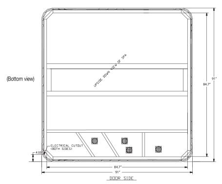
**NOTE:** Watkins Manufacturing Corporation recommends that the Tobago be installed on a minimum 4" thick reinforced concrete pad or structurally sound deck able to support the "dead weight" found in the spa specification chart.
