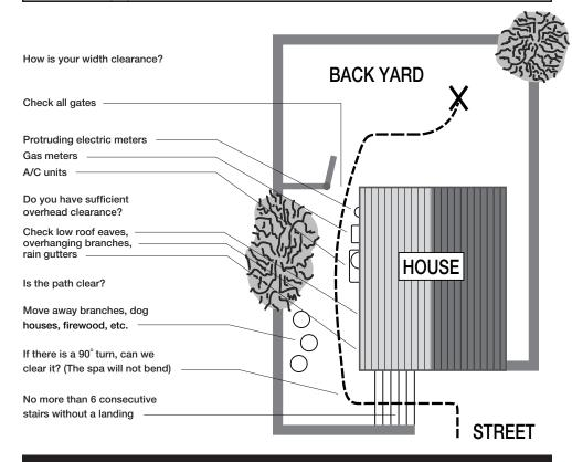
It may be necessary to remove a gate, part of a fence, or other movable obstructions in order to roll the spa to its installation site. About ten percent of the time, a crane is the only way to install the spa by lifting it to its final destination.
