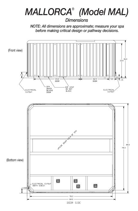
**NOTE:** Watkins Manufacturing Corporation recommends that the Mallorca be installed on a minimum 4" thick reinforced concrete pad or structurally sound deck able to support the "dead weight" found in the spa specification chart.
