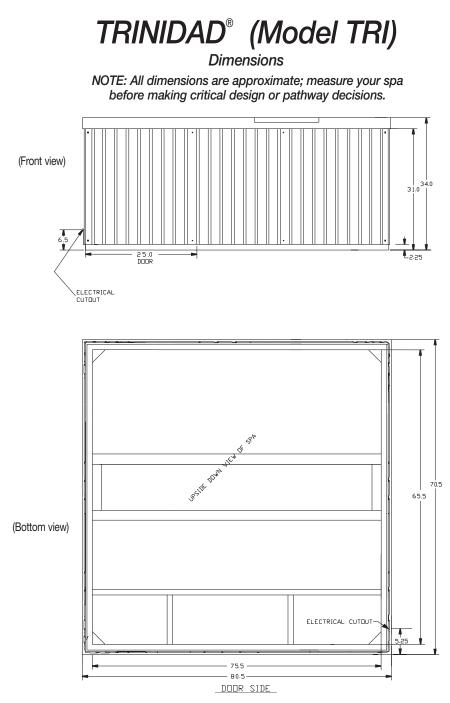
**NOTE:** Watkins Manufacturing Corporation recommends that the Trinidad be installed on a minimum 4" thick reinforced concrete pad or structurally sound deck able to support the "dead weight" found in the spa specification chart.
