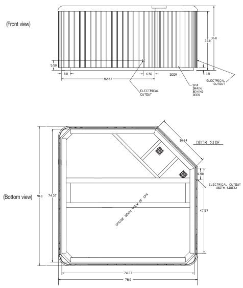
**NOTE:** Watkins Manufacturing Corporation recommends that the Sorrento be installed on a minimum 4" thick reinforced concrete pad or structurally sound deck able to support the "dead weight" found in the spa specification chart.
