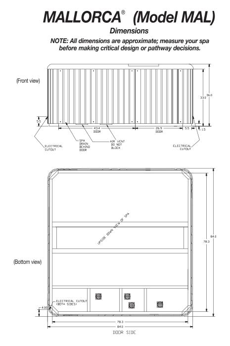
**NOTE:** Watkins Manufacturing Corporation recommends that the Mallorca be installed on a minimum 4" thick reinforced concrete pad or structurally sound deck able to support the "dead weight" found in the spa specification chart.
