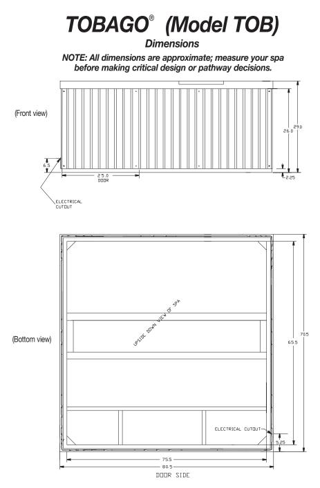
**NOTE:** Watkins Manufacturing Corporation recommends that the Tobago be installed on a minimum 4" thick reinforced concrete pad or structurally sound deck able to support the "dead weight" found in the spa specification chart.
