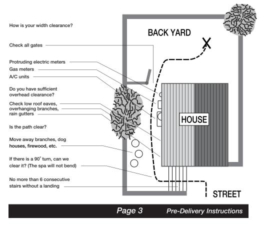
It may be necessary to remove a gate, part of a fence, or other movable obstructions in order to roll the spa to its installation site. About ten percent of the time, a crane is the only way to install the spa by lifting it to its final destination.
