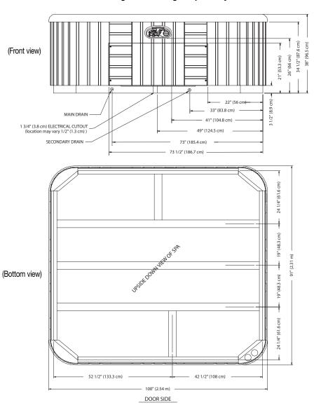
**NOTE:** Watkins Manufacturing Corporation requires that the Vista be installed on a minimum 4" thick reinforced concrete pad or a deck that is able to withstand more than 115 lbs. per square foot.
