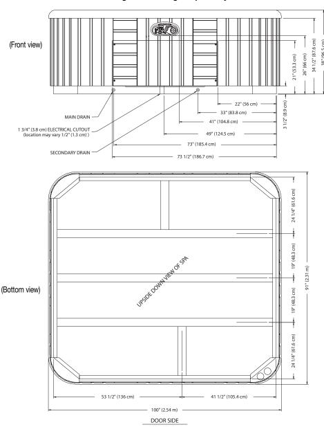
**NOTE:** Watkins Manufacturing Corporation requires that the Grandee be installed on a minimum 4" thick reinforced concrete pad or a deck that is able to withstand more than 115 lbs. per square foot.
