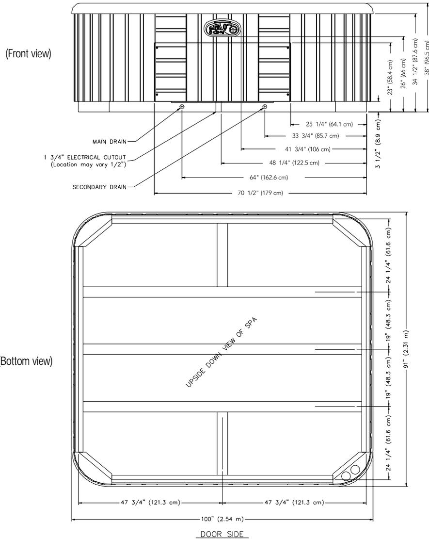
**NOTE:** Watkins Manufacturing Corporation requires that the Landmark® be installed on a minimum 4" thick reinforced concrete pad.
