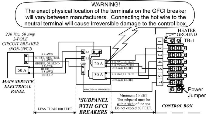
**NOTE:** The wire connections to G.F.C.I. breakers are for reference only. Always ensure the white neutral wire is connected to the load neutral of the 20 amp breaker.
