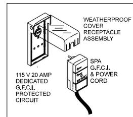
All 230 volt Hot Spring® Spas must be wired in accordance with applicable local electrical codes, and all electrical work must be done by a licensed electrician.
