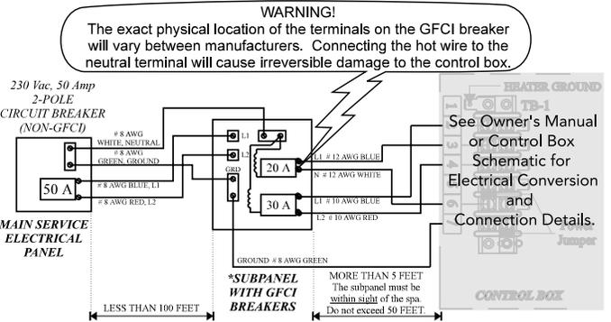
**NOTE:** The wire connections to G.F.C.I. breakers are for reference only. Always ensure the white neutral wire is connected to the load neutral of the 20 amp breaker.
