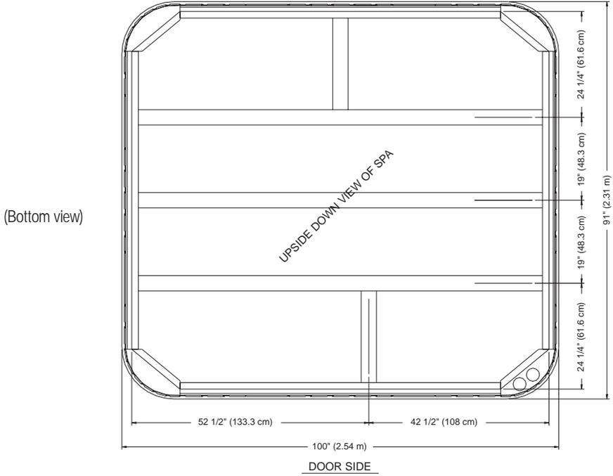
**NOTE:** Watkins Manufacturing Corporation requires that the Landmark be installed on a minimum 4" thick reinforced concrete pad.
