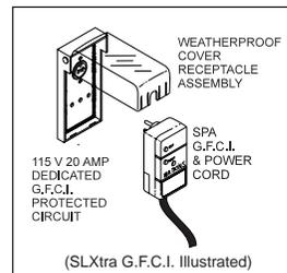
All 230 volt Hot Spring® spas must be wired in accordance with applicable local electrical codes, and all electrical work must be done by a licensed electrician.
