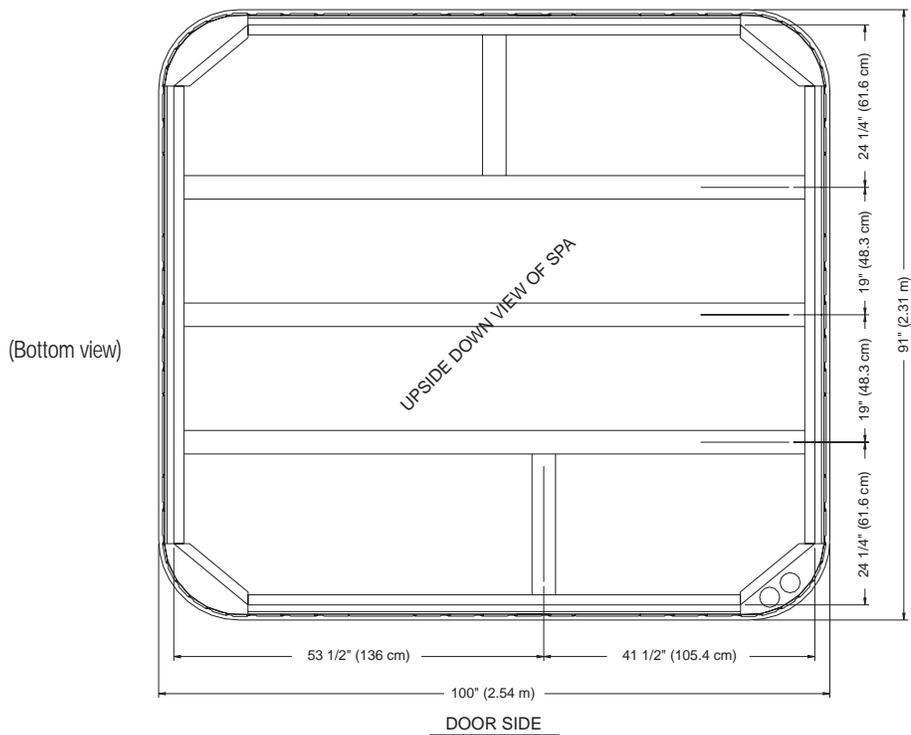
**NOTE:** Watkins Manufacturing Corporation requires that the Grandee be installed on a minimum 4" thick reinforced concrete pad.
