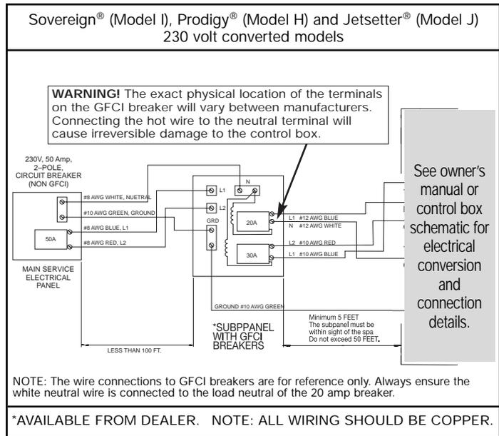
See owner's manual or control box schematic for electrical conversion and connection details.
